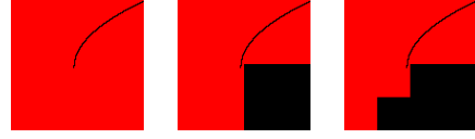
Figure 6: A sequence of computed graphs, from procedure 1, of y < \sqrt{x} over [-1, 1.1] \times [-1, 1.1] with an 8 \times 8 pixmap; the thin black curve shows the true graph of y = \sqrt{x} . The computed graph on the right is incorrect.
